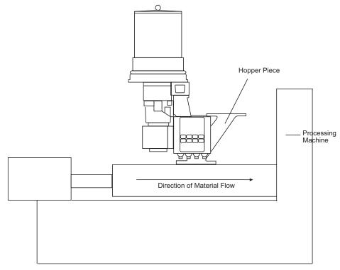
Figure 4. Digital Dosing Feeder Assembly
